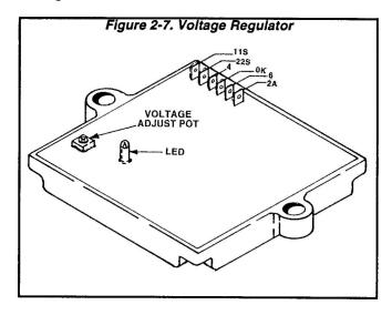
NOTE: Adjustment of the regulator's "VOLTAGE ADJUST" potentiometer must be done only when the unit Is running at Its correct governed no-load speed. Speed Is correct when the unit's no-load AC output frequency Is about 61-63 Hertz. At the stated frequency, AC output voltage should be about 122-12 volts.
