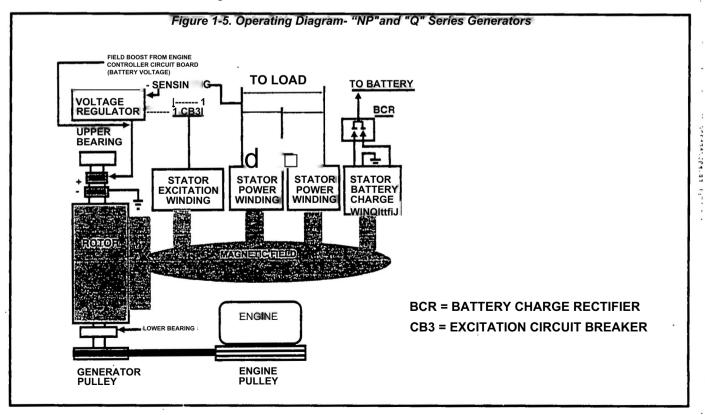
(1) If the actual (sensing) voltage Is greater than the pre-set reference voltage, the Regulator will decrease the regulated current flow to the Rotor.
