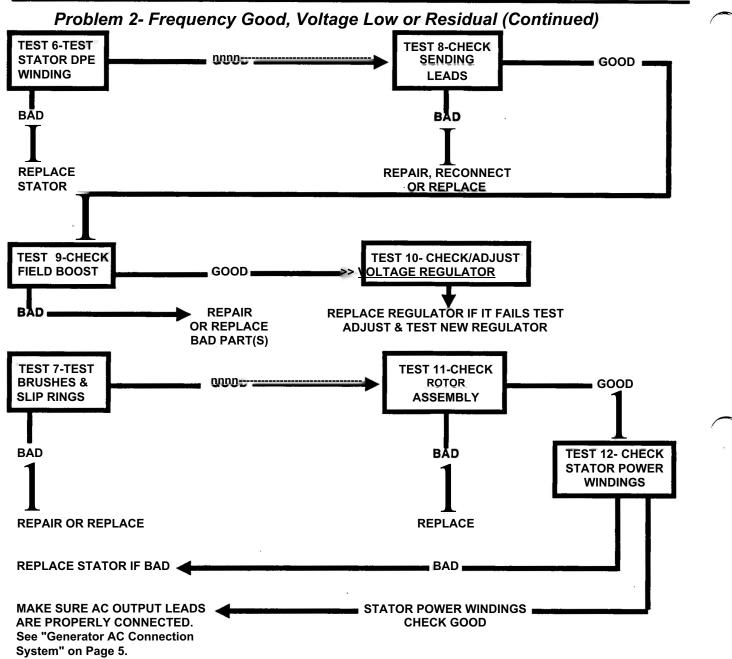
NOTE: The term "Low Voltage" refers to any AC output voltage that Is less than rated voltage. The term "Residual Voltage" refers to AC output voltage produced by Rotor residual magnetism alone and without excitation current (about 5-12 volts AC).
