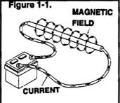
From the above, it is clear that the stronger the magnetic field the greater the voltage induced into the conductor. Additionally, it is apparent that the greater the current flow through the conductor the stronger the magnetic field around that wire. The following rules then apply:
