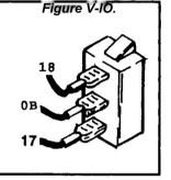
A defective Start-Stop Switch can result In (a) failure to crank and/or (b) failure to shut down when the Switch Is set to "STOP".
