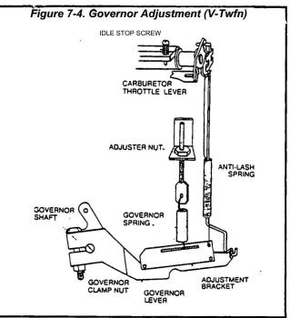
a. Inspect the ANTI-LASH SPRING. Make sure It Is not broken or disengaged.
