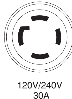
Figure 12 - 120/240 VAC, 30 Amp Receptacle
