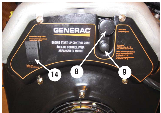
Figure 6 - Engine Control Panel
