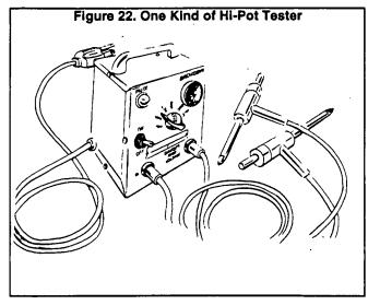
To measure Insulation resistance, connect one tester lead to the leads for the winding to be tested and the other tester lead to the generator frame. Make sure no leads of the part being tested are touching any metal parts of the generator. If the 'Neutral' is grounded, it must be disconnected. Follow the tester manufacturer's instructions and perform the resistance test.
