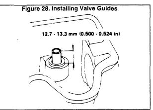
4. Heat the cylinder head to 302°-320° F. (150°-160° C.), then press service valve guide onto cylinder head (see Figure 28).
