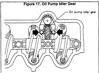
1. Remove timing belt (Section 2.2). Then, remove OIL PUMP IDLER GEAR.
