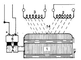
The VOLTAGE REGULATOR will continue to increase or decrease direct current flow to the ROTOR, In an attempt to maintain STATOR AC POWER WINDING voltage at the same value as the REGULATOR'S preset REFERENCE voltage.
