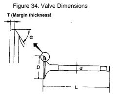
NOTE: When the valve head Is worn to 0.020Inch (0.5mm) margin thickness, replace the valve. Grinding allowance for valve stem end surface Is 0.008 Inch (0.2mm) or less.
