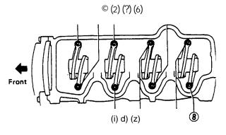
4. When valve clearances are properly set, tighten the adjusting screw locknut to 8-11 foot-pounds (11-15 N-m).
