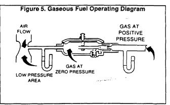
The following facts apply to venturi type gas carburetion systems:
