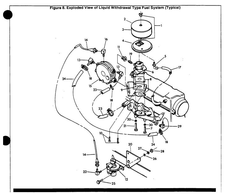
Parts List for Liquid Withdrawal Fuel System
