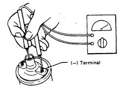
Checking the Condenser Use a capacity tester to check the condenser. If a capacity tester is not available, avolt-ohm-milliammeter(VOM) may be used to test the condenser, as follows:
