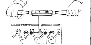
3. Ream the cylinder head's valve guide hole (Figure 27).
