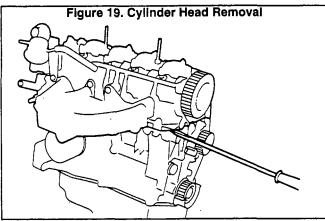
3. If the cylinder head is difficult to separate, pry with a screwdriver.
