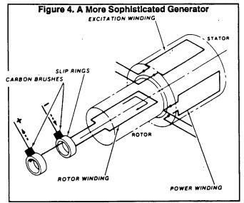
A Typical AC Generator Rgure 5, below, Is an operating diagram of a typical AC generator. Operation of this typical generator may be briefly described as follows:
