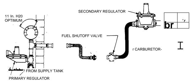
Figure 2. A Typical Vapor Withdrawal System
