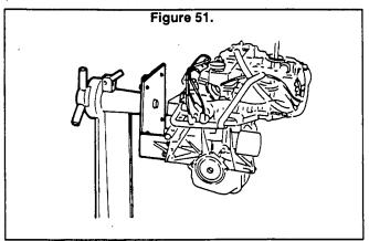
2. Remove crankshaft rear oil seal retainer. Remove bearing caps. Remove the crankshaft.
