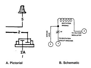
Figure 33. Thermal Protector Bypassed
