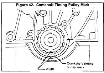
CAUTION: DO NOT rotate crankshaft and camshaft separately or valves will hit the piston heads. 2. Install cylinder head with a new gasket. The following rules apply:
