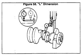
7. Check crankshaft runout. "T.I.R." stands for "Total Indicator Reading".
