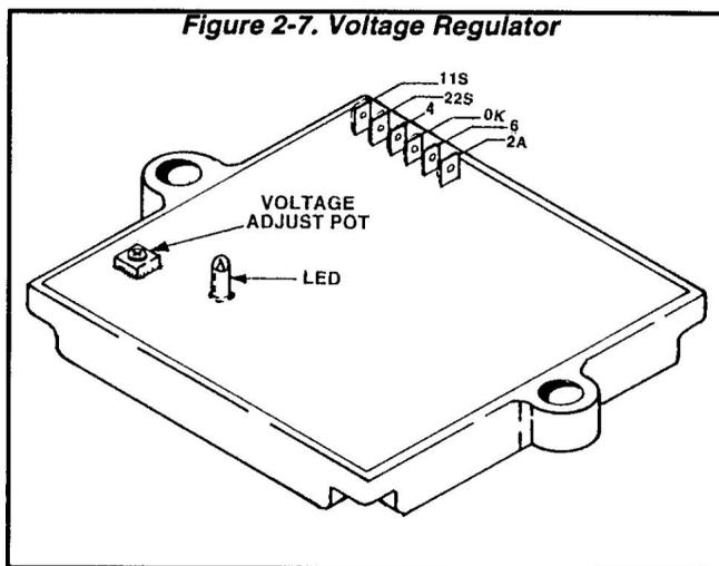
**NOTE:** Adjustment of the regulator's "VOLTAGE ADJUST" potentiometer must be done only when the unit is running at its correct governed no-load speed. Speed is correct when the unit's no-load AC output frequency is about 61-63 Hertz. At the stated frequency, AC output voltage should be about 122-127 volts.
