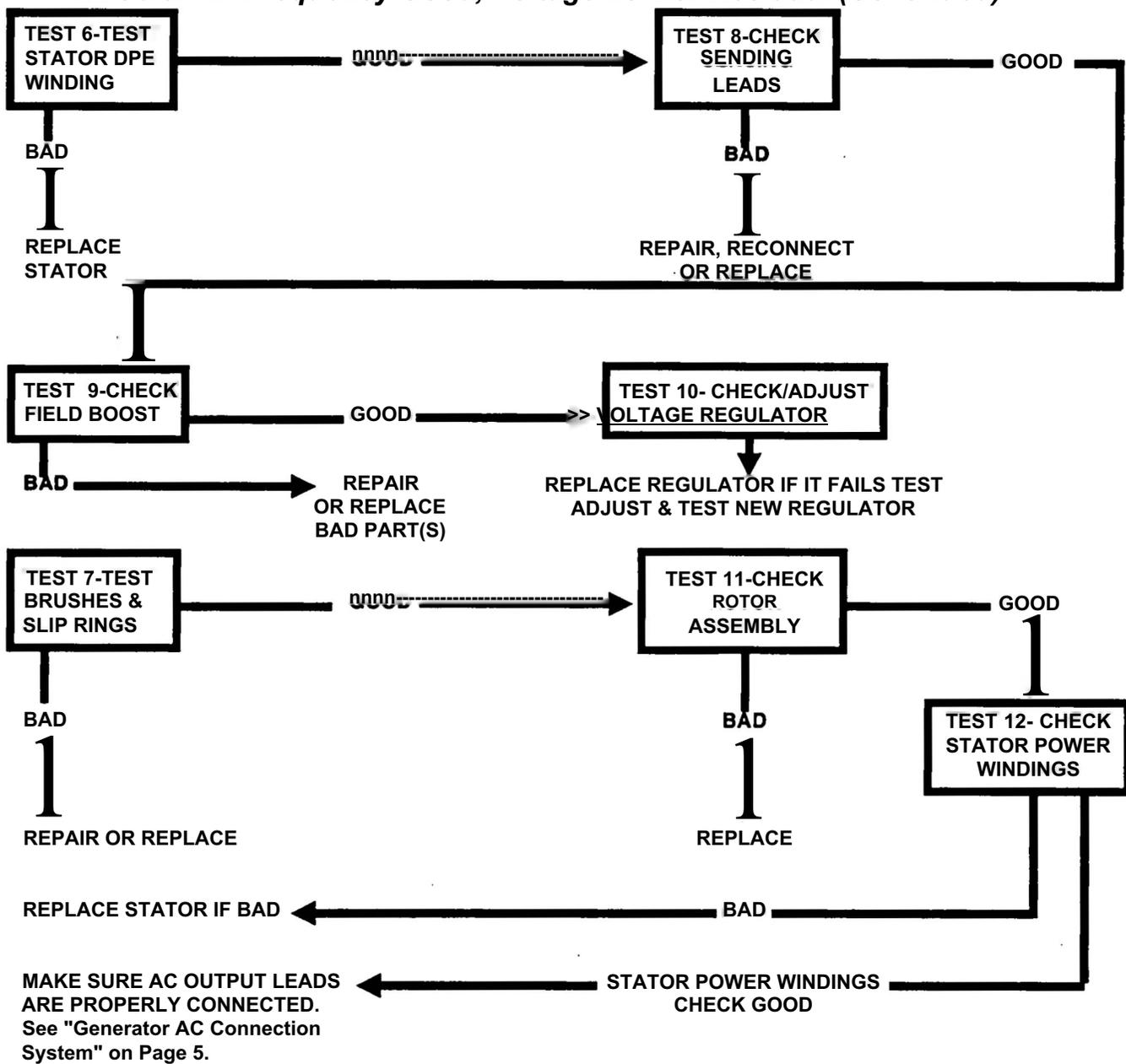
NOTE: The term "Low Voltage" refers to any AC output voltage that is less than rated voltage. The term "Residual Voltage" refers to AC output voltage produced by Rotor residual magnetism alone and without excitation current (about 5-12 volts AC).
