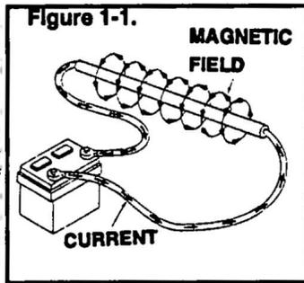
From the above, it is clear that the stronger the magnetic field the greater the voltage induced into the conductor. Additionally, it is apparent that the greater the current flow through the conductor the stronger the magnetic field around that wire. The following rules then apply:
