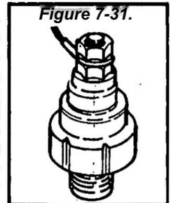
If the switch falls closed, the engine will crank and start but will then shut down after a few seconds.
