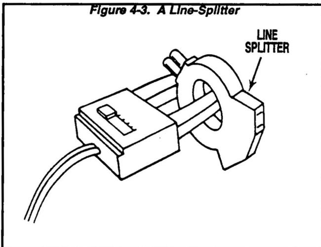
**NOTE:** If the physical size of the conductor or ammeter capacity does not permit all lines to be measured simultaneously, measure current flow in each individual line. Then, add the individual readings.
