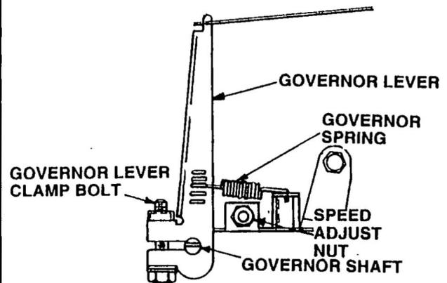
Figure 7-6. Carburetor Adjustment (GN-360 Engine)
