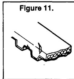
**NOTE:** Replace the timing belt if (a) side surface is worn to such an extent that cutoff performed during the manufacturing process cannot be seen, (b) belt corners are worn or rounded, or (c) belt fibers are frayed and coming out.
