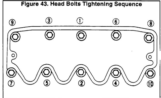
3. Tighten cylinder head bolts as follows:
