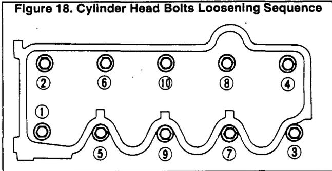
2. Remove the cylinder head. Loosen bolts in 2 or 3 stages, in the sequence shown above.
