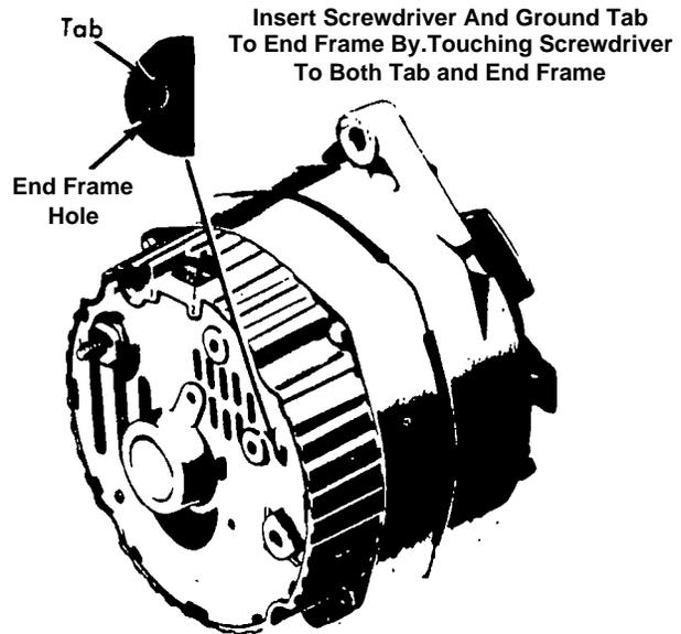
Figure 5. DC Alternator Test Connections
