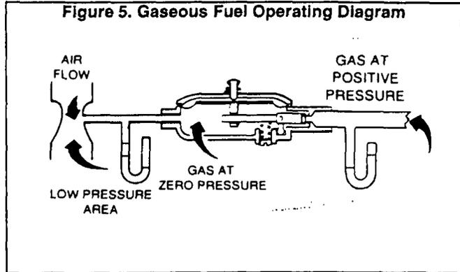
The following facts apply to venturi type gas carburetion systems:
