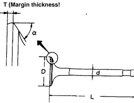
**NOTE:** When the valve head is worn to 0.020 inch (0.5mm) margin thickness, replace the valve. Grinding allowance for valve stem end surface is 0.008 inch (0.2mm) or less.
