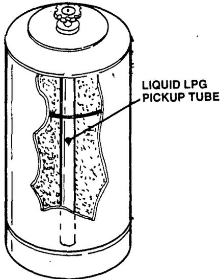
Figure 4. Typical Liquid Withdrawal Fuel System
