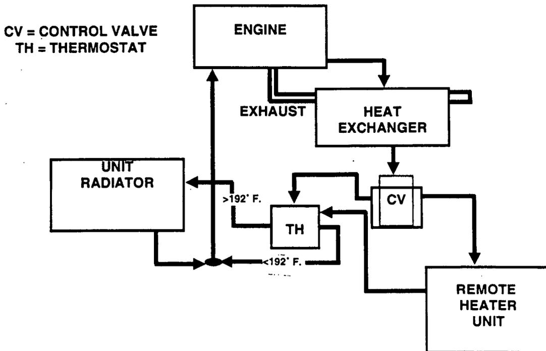
Figure 12. Exploded View of Heat Recovery System
