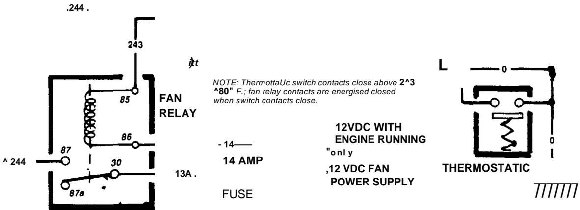
Figure 10. A Remote Radiator, Fan and Wiring Harness
