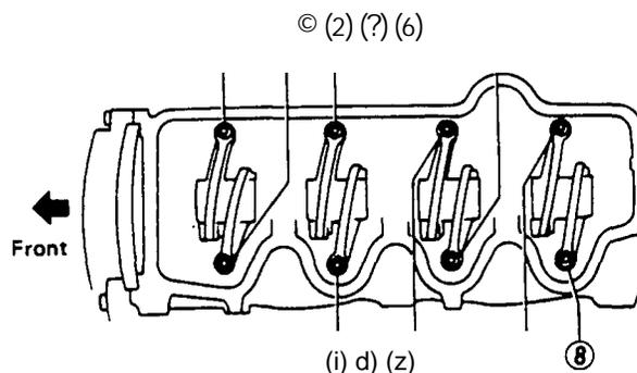
4. When valve clearances are properly set, tighten the adjusting screw locknut to 8-11 foot-pounds (11-15 N-m).
