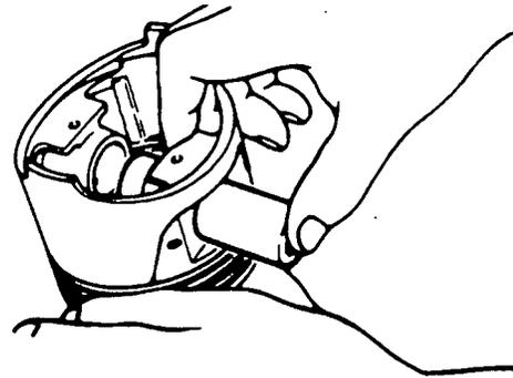
Figure 54. Ring-to-Groove Side Clearance
