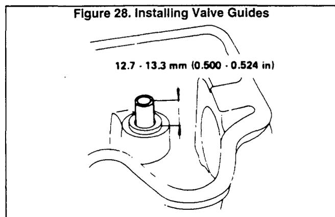
4. Heat the cylinder head to 302°-320° F. (150°-160° C.), then press service valve guide onto cylinder head (see Figure 28).
