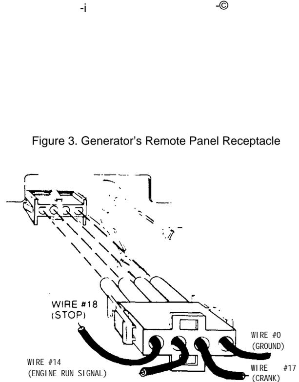
Figure 3. Generator's Remote Panel Receptacle
