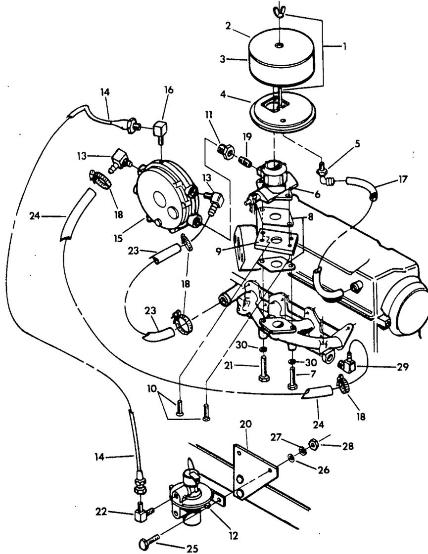
Parts List for Liquid Withdrawal Fuel System
