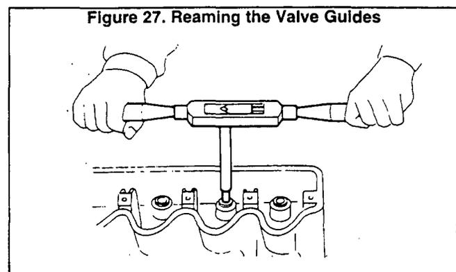
3. Ream the cylinder head's valve guide hole (Figure 27).
