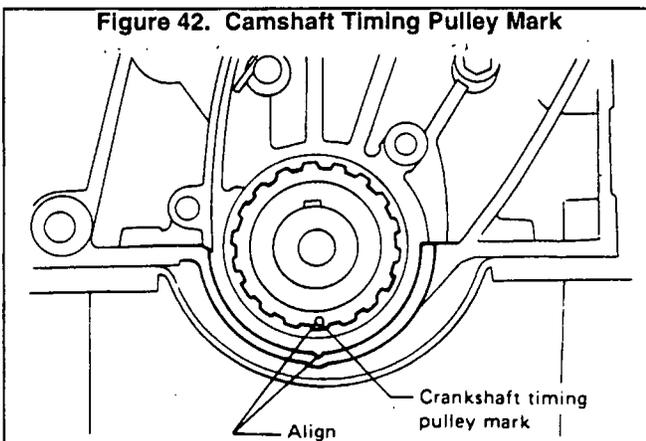
**CAUTION: DO NOT** rotate crankshaft and camshaft separately or valves will hit the piston heads.
